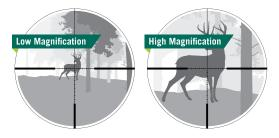
**Note:** The Viper<sup>®</sup> HD 5-25x50 SFP riflescope's reticle is calibrated to 20x. For a hashmark's value to be true, it would need to be used on 20x. There will be a detent on the magnification ring at 20x.
